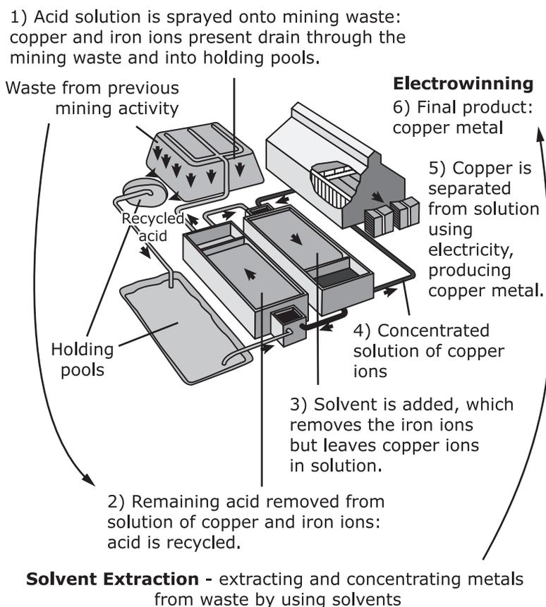
**Figure 1. Solvent Extraction and Electrowinning of Copper**
